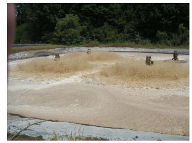
with a vengeance: alkalinity addition had been increased and maintained at maximum levels; the resultant intermittent excursions in pH levels combined with nutrient overdosing were causing demonstrable incidences of toxicity and inhibition.
